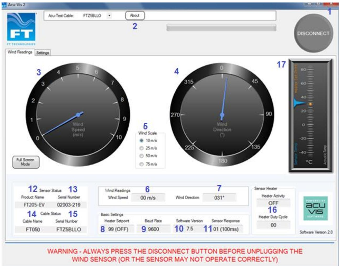
Acu Vis Main Display – Connected to a FT205 Wind Sensor
